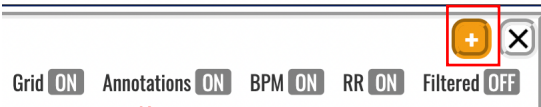
Figure 116: Tools in the header of the extended viewer and the "Add to report" button.
